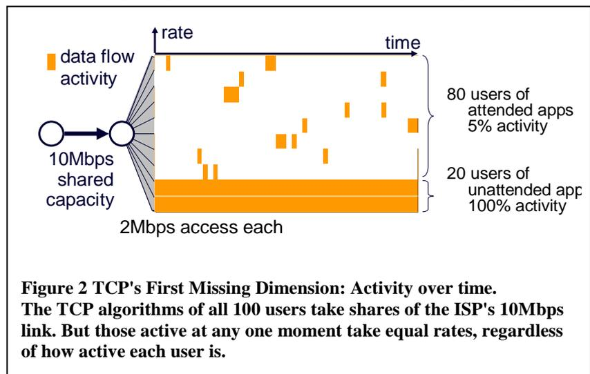
**Figure 2** TCP's First Missing Dimension: Activity over time. The TCP algorithms of all 100 users take shares of the ISP's 10Mbps link. But those active at any one moment take equal rates, regardless of how active each user is.
