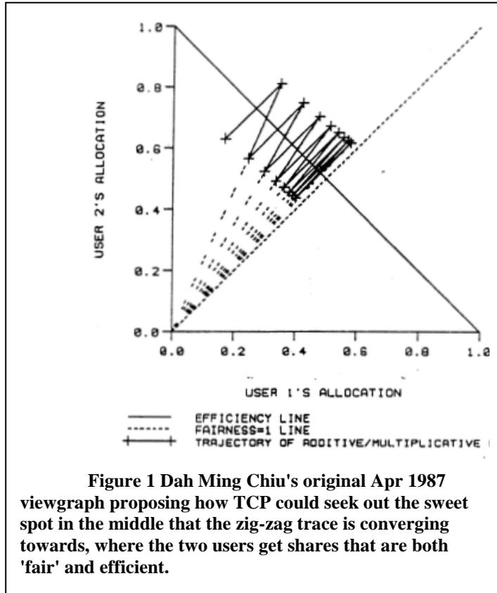
**Figure 1** Dah Ming Chiu's original Apr 1987 viewgraph proposing how TCP could seek out the sweet spot in the middle that the zig-zag trace is converging towards, where the two users get shares that are both 'fair' and efficient.
