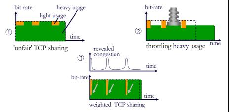
**Figure 3**—Throttling (2) makes light usage a little faster by slowing down heavy users. Whereas weighted TCP sharing (3) allows light usage to go much faster, hardly affecting heavy users.
