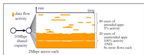
Figure 2—TCP's Second Overlooked Factor: Multiple TCP Instances.
